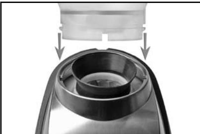
To replace the bean hopper, line up the two small tabs on the base of the hopper with their respective slots in the top of the grinder housing and insert the hopper into the grinder. Once the hopper is in place rotate it clockwise to your desired grind setting.
