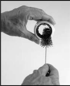
Use the bristle brush (included with your grinder) to remove any loose coffee residue on the ring burr and the center cone burr mounted within the motor housing. Wash the silicone seal in warm soapy water and dry.
