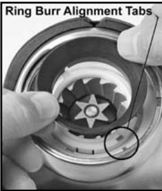
Ensure that the red tab on the adjustment ring located inside the top of the grinder housing is positioned as shown in the picture at left. If the red tab is not in the correct position, turn the adjustment ring counterclockwise as far as it will go. Replace the burr by lining up the red tab on the burr with the red tab on the adjustment ring. Wiggle and push down firmly on the ring burr to ensure that it seats properly.
